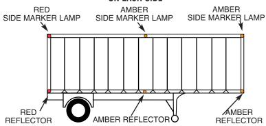
Intermediate side marker lamp and reflector required only on trailers measuring 30 feet or more in length.
