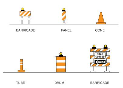
The diagonal stripes on the barricade or vertical panel guide the driver towards the direction to which the traffic is to pass. Stripes sloping downward to the right mean the driver should bear to the right. Conversely, stripes sloping downward to the left mean bear to the left.
