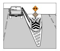
Barrels engineered to act as an impact cushion is a new concept in reducing the seriousness of crashes. These barrels are usually installed in front of a solid obstacle and at an area of high crash frequency.
