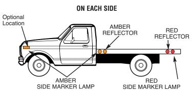
\*Trucks manufactured or assembled prior to model year 1960 required to have at least one taillight.
